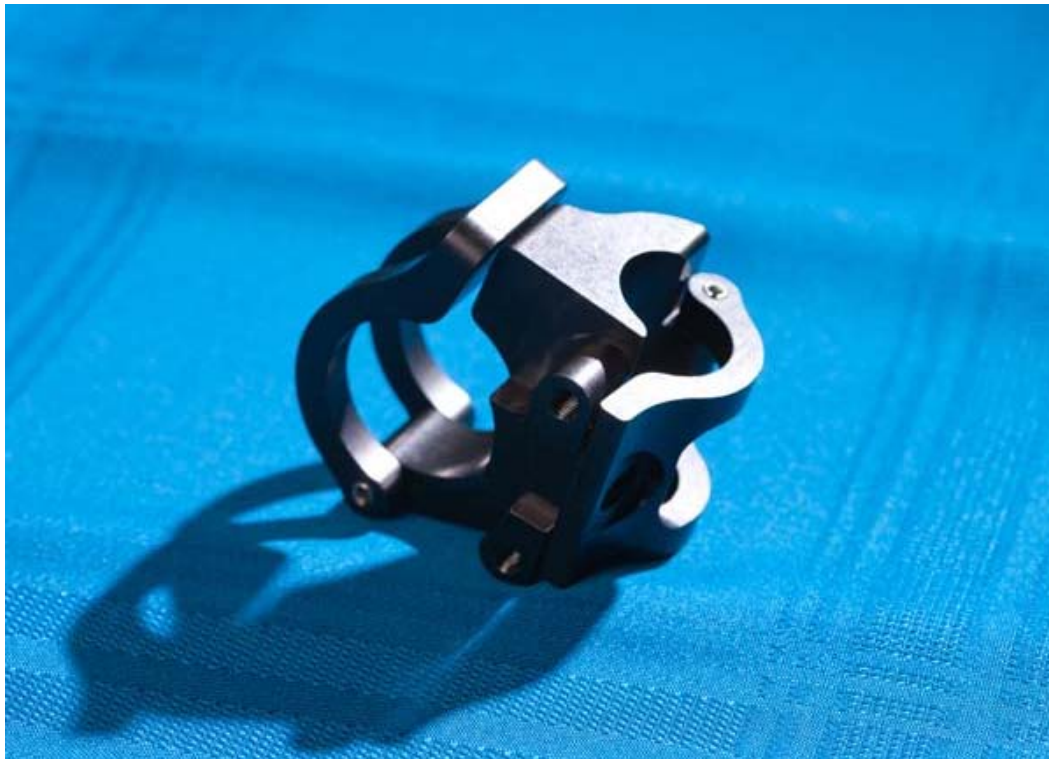
A camber clamp assembly, manufactured by Alexandria Industries for use on a wheelchair. The assembly illustrates the versatility of aluminum extrusion combined with hardcoat anodizing, a combination that helps prevent corrosion and chemical absorption and eases the cleaning process in medical care applications. Photo courtesy of Alexandria Industries.
